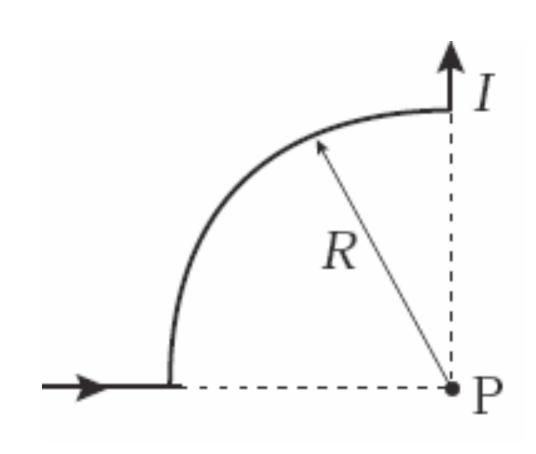
The segment of wire (total length = 6R) is formed into the shape shown and carries a current I. What is the magnitude of the resulting magnetic field at the point P?
