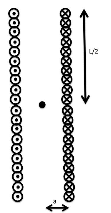
Magnetic field at the center of the solenoid
